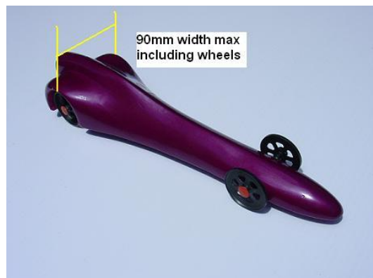
(E) Dragster Body Width (including wheels)
