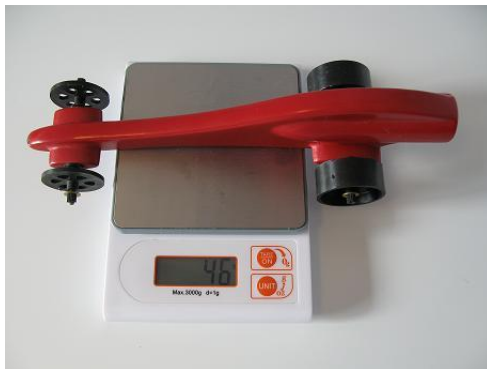
(C) Dragster body mass /weight with wheels No Co2 cartridge
